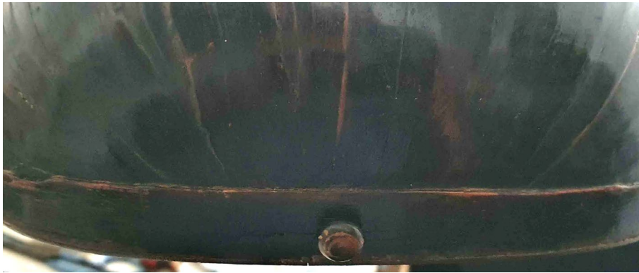
PLATE 1. A black 18 th century instrument showing surface coating worn through to the sealed bare wood beneath.
