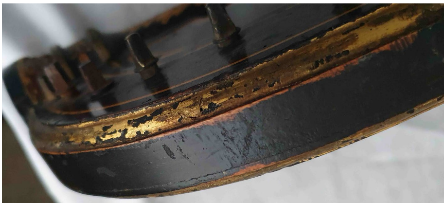
PLATE 2. Part of a 19 th century instrument showing surface coating worn through on the edges.
