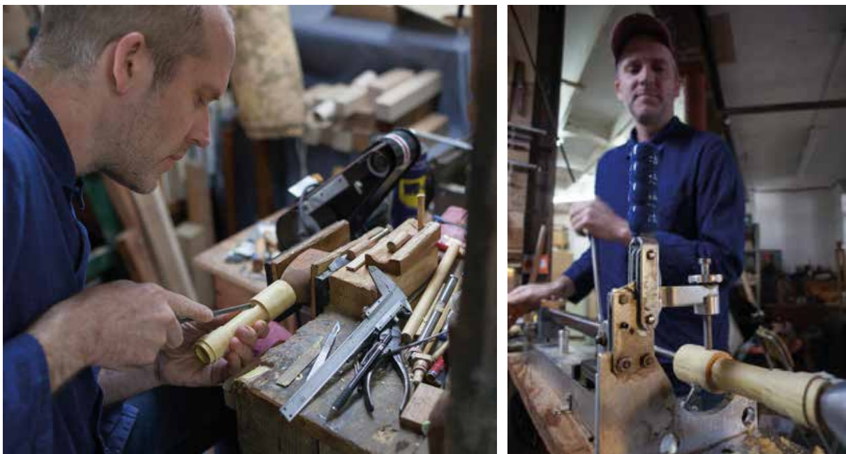
Left: Working on the head section, right: reaming part of the head chamber
