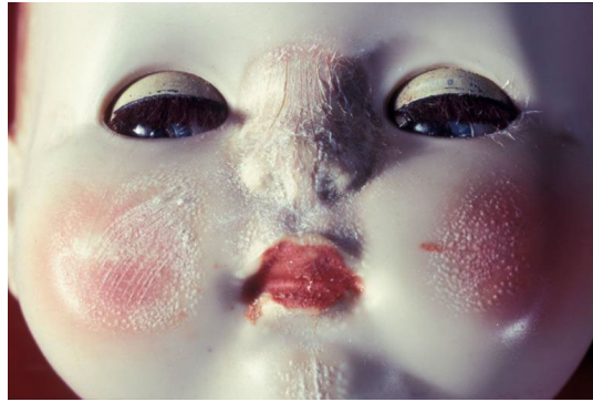
PLATE 7 : This cellulose acetate doll's face has suffered due to plasticiser out-migration and acetic acid vapours generated from the chemically degrading material itself 14 .
