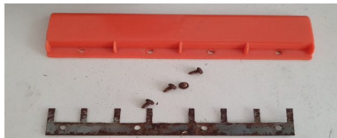
PLATE 2: Keybox cover and sheet steel spring bar with its 'teeth' springs
