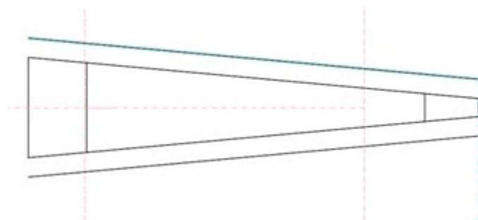
In the following images we can see the constraints set on the model. For example, the total width of the Pegbox 1 at the lower block is 63mm and the inner height is 157mm. These constraints we shall vary per pegbox, whereas other constraints are fixed, such as the pegbox cheeks being set to 9mm, and the inner width at the top of the pegbox being 13mm.
