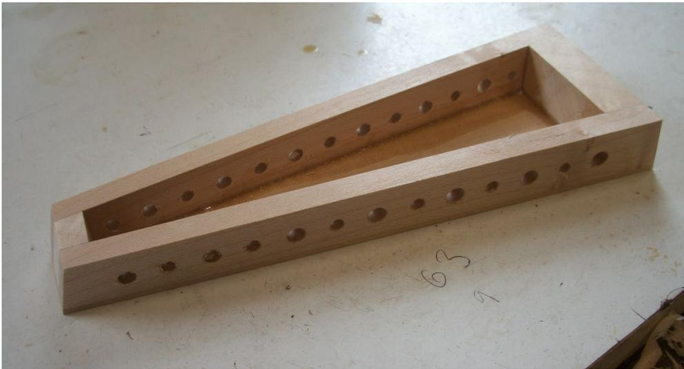
Each pegbox is unique to that model of lute – the dimensions are more or less pre-determined by other dimensions and features of the instrument:
