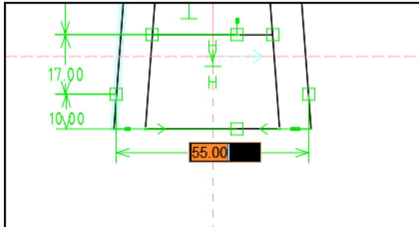
In Pegbox 2 we use the same model to derive a design for a pegbox for a 55mm slot and a 145mm inner length. Other dimensions are unaffected such as the length of the legbox blocks or the width of the pegbox cheeks.
