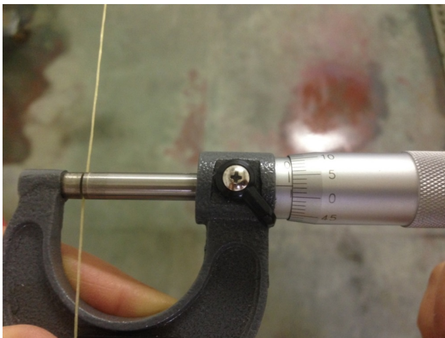
Measurement carried out on the opposite end of the dried 7.2 m string: 0.52 mm unpolished
