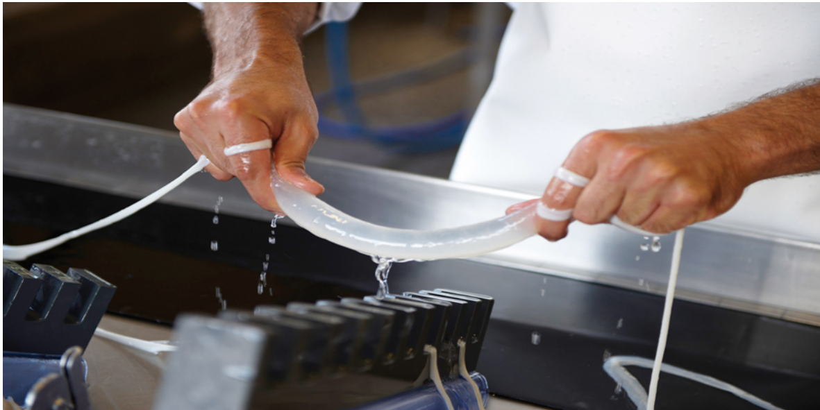
Variable gauge to determine the diameter of the gut
