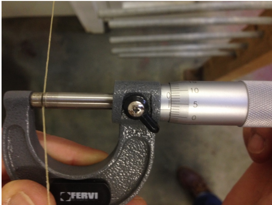
Measurement carried out on one end of the dried string of 7.2 m: 0.53 mm unpolished
