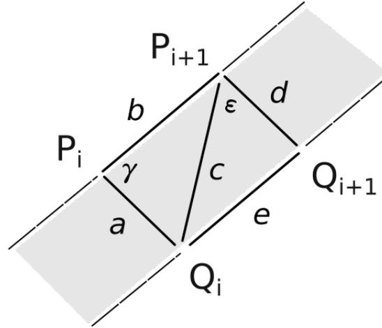
**Figure 3.** Definition of conserved lengths exploited by the multi-rib algorithm
