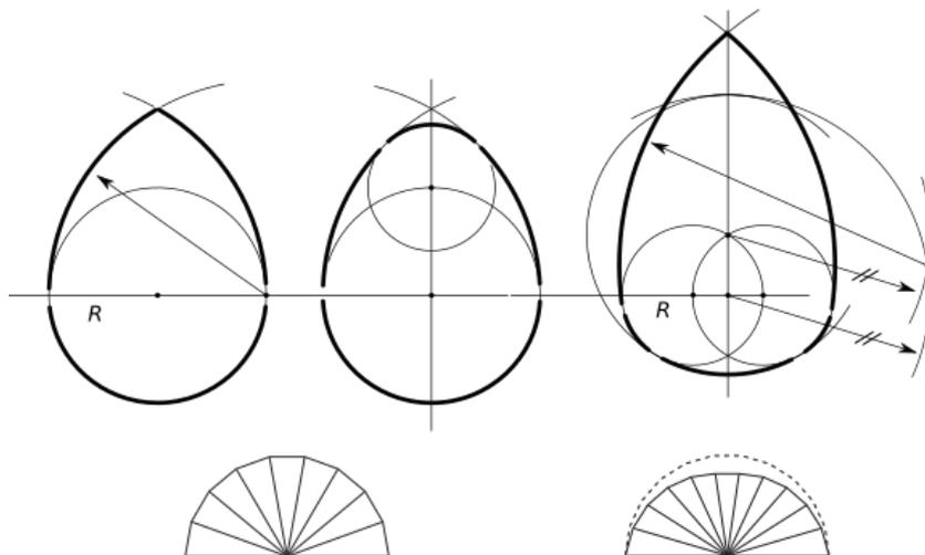
**Figure 1.** Belly elevations generated with compass and straight edge from a fiducial radius  $R$ , with associated seam structures in axial elevation. (L to r) 13th century Arabic; Arnaut de Zwolle (15th century); Magno Tieffenbrucker (1609)
