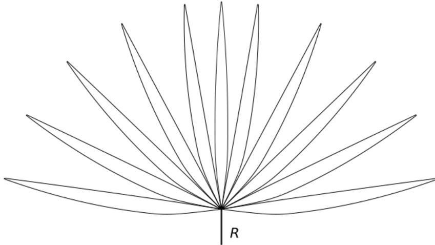
**Figure 2.** Algorithmically computed stencil map for the flattened-back 11-rib Tieffenbrucker bowl. Depth 143mm, breadth 353mm Cepelak (1999) ( $\delta = 0.22$ ). The stem is the belly fiducial radius marked in Fig.1.
