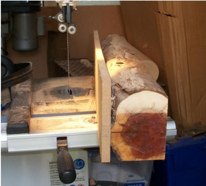
Rotate the log up and onto this cut face, and now we can use the board against the fence to cut a square line, again well aligned into the log.
