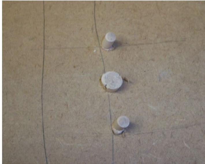
Now mark a reference line a fixed distance from the edge or centre of the log. This will depend on whether you want the cut to align with the edge or centre of the log.
