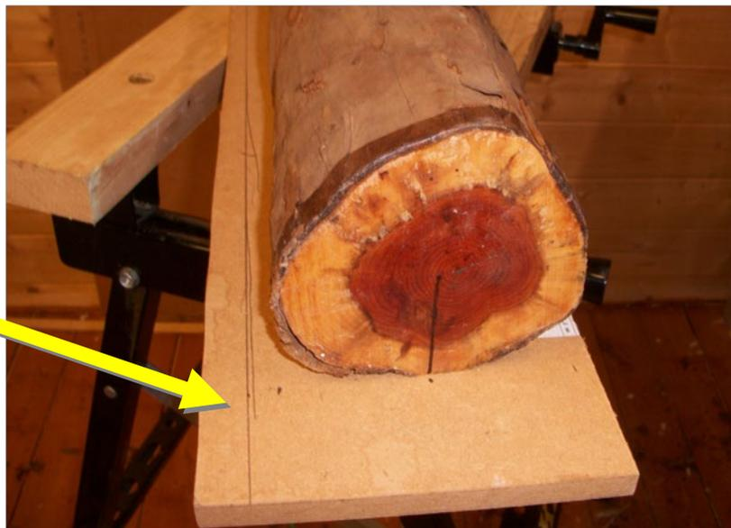
Place the assembly onto your saw table and cut by eye along the reference line.
