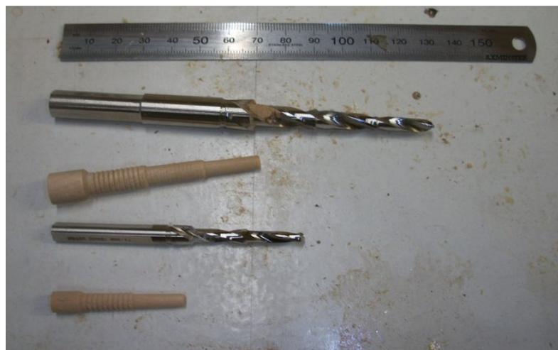
Instead I am using an engineered stepped dowel system – called “Miller Dowel”<sup>1</sup> which comes with a convenient cutting bit that precisely fits the shape of the dowel. Three sizes are available, the most useful being the ones approximately 40 and 70mm long.
