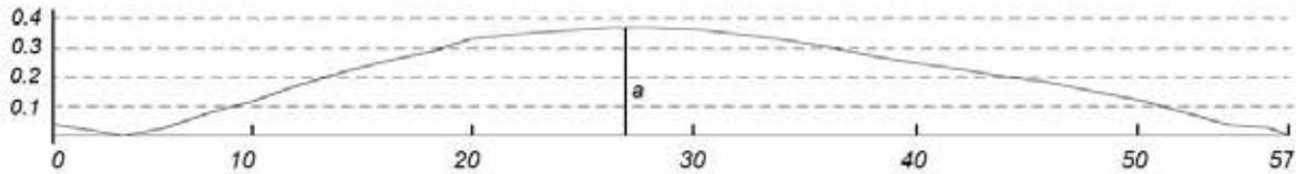
It happens that the highest point of the graph is just at L 27 (a), with a value of 0.37 mm. But as we have seen that from L 27 onwards the windway roof is parallel to the axis of the head, in the diagram below I have tilted the graph until the line after L 27 almost running horizontally to the right. And now it becomes clear that the windway roof is sharply rising from (close to) the beginning up to about L 27.
