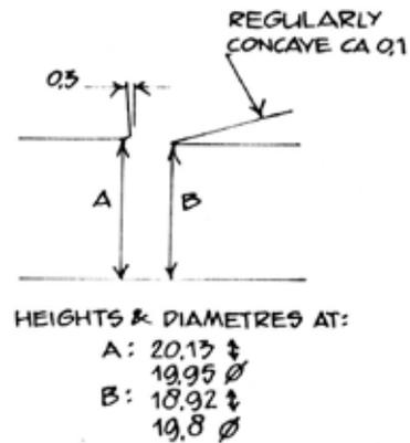
Another decision of Hans Schimmel and Rob van Acht was the choice of data they gave for the fingerholes. They measured the smallest size (Y) in two directions, and the dimensions, also in two directions at the surface of the wood. But they didn't give data for the undercutting of the holes. As they explained: these measurements are not accurate enough.
