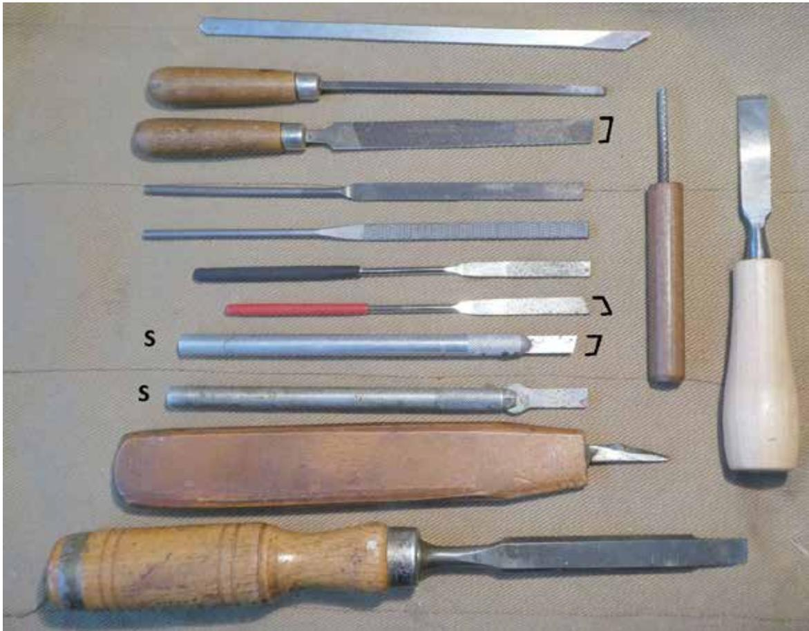
A selection of tools for shaping and finishing the window and labium: small knives, chisels, rasps, files and scrapers (S). I have ground some of the tools with an oblique angle, so that they fit better in the corners of the labium (for instance the side walls); see the marks on the photo. When cutting the labium with a chisel, I put a small piece of wood in the window to avoid damage at the north face of the window (photo, right).
