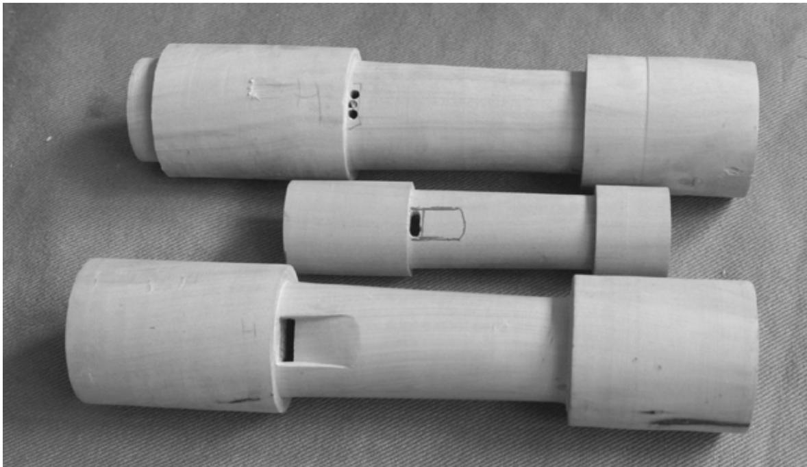
Three phases of making a window and labium in a ‘working head’.
