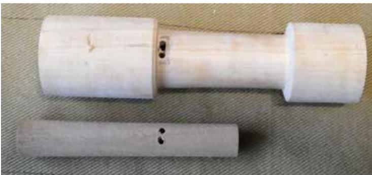
Left: the wooden plug (here taken out) used for filling the bore in the section of windway prevents the wood splintering when the drill goes through the wall into the bore of the head.
