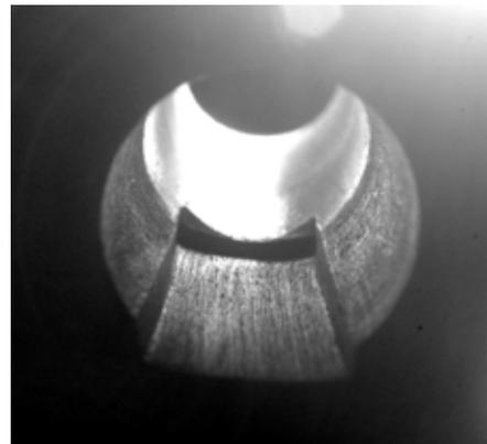
Photo right: the much shorter candle flame in the head of one of my (still unfinished) recorders. The windway roof is here in much better condition, but the sidewalls of the windway are still a bit sloppy.
