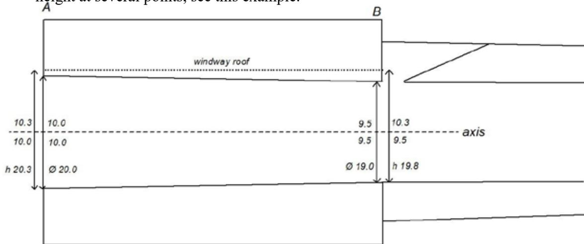
It is for an alto recorder, with a windway parallel to the axis, and with a step of 0.8 mm. The bore diameter at A is  $\text{Ø } 20.0$  mm, at B and C 19.0 mm. We have to do now some calculations. A step of 0.8 means that at point B the height must become 19.8 mm, that is from the roof to the axis  $19.8 - 9.5 = 10.3$  mm.
