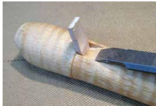
2- Making the windway (first phase), with hand tools or a windway cutting machine.
