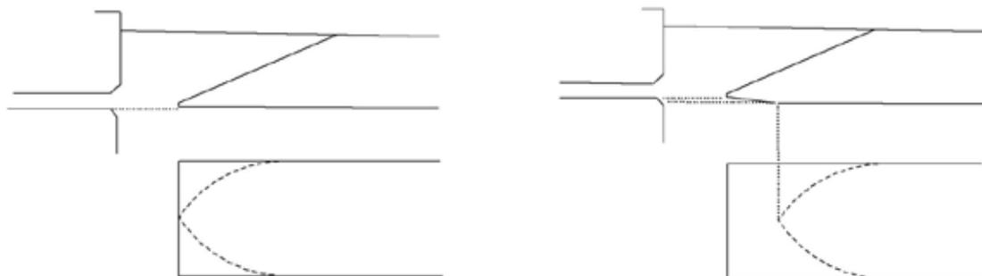
On the left diagram: candle flame with its top reaching the labium edge. On the right diagram: the labium is undercut over some millimeters. It is a way to make the step which is too big a bit smaller.
