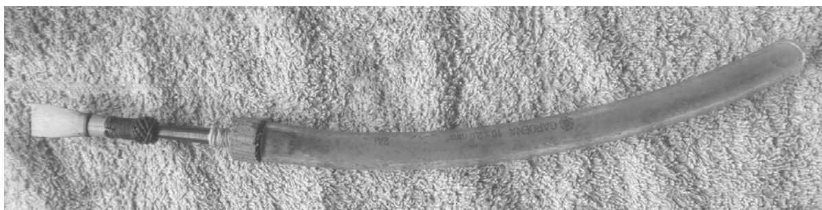
Fig. 5: bassoon reed on a plastic tube (internal diameter 10 mm, length c. 190 mm)
