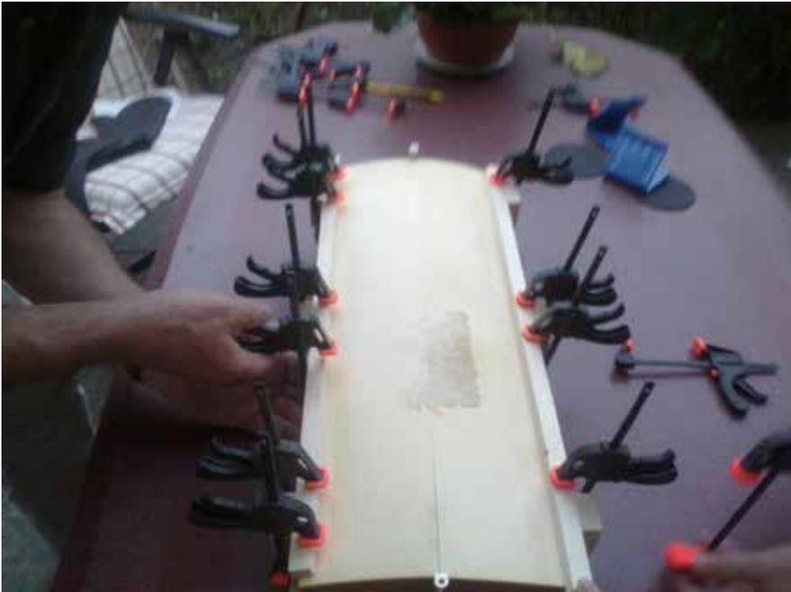
As you can see the glued seam parted in the middle. So, this was not the way to bend the top plate!
