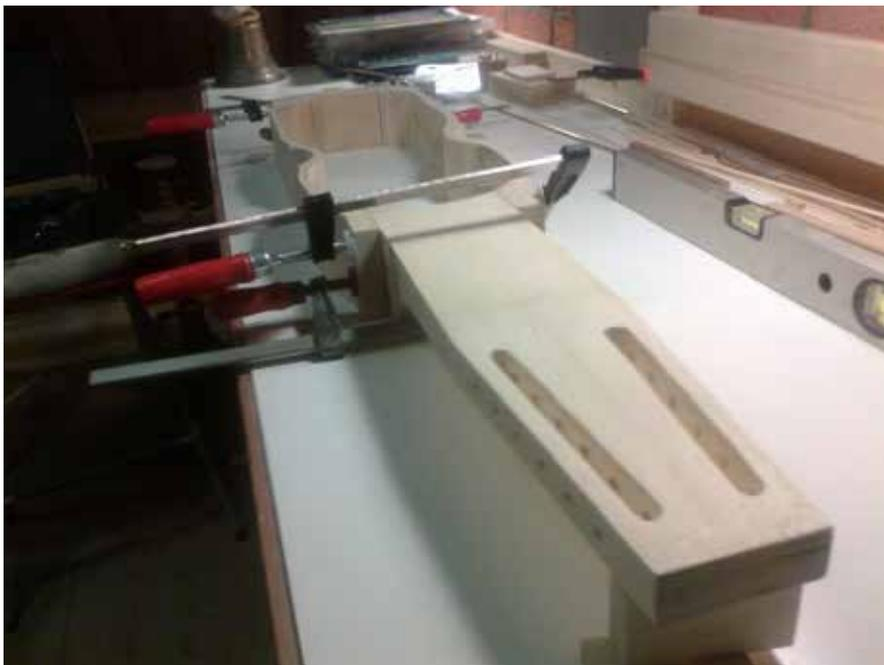
Here you can see how the parts are glued together and clamped. After this was done, I glued and clamped the back to the harpa.
