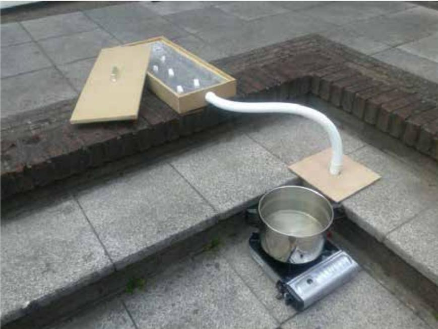
After 15 minutes steaming the top plate could be bent and clamped to the mould that I created earlier.
