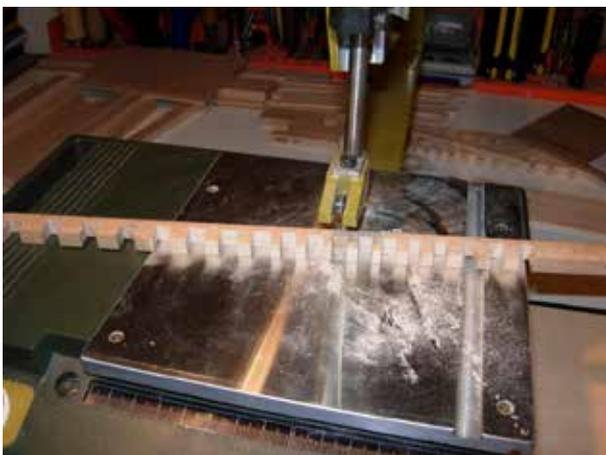
Finally, I covered the inside of the teeth of the key guides with supple leather of 1 mm thickness. (This means that where the keys slide through the key guides; the keys should be 1 mm less thick than is indicated in the construction manual).
