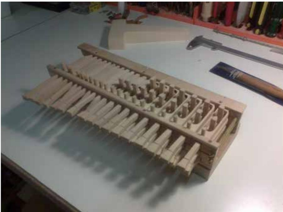
Because key guides remained not exactly vertical, I made cross connections between the left and right key guides. They consist of threaded rod that runs through the key guides. For show, I caught the rod in a brass tube.
