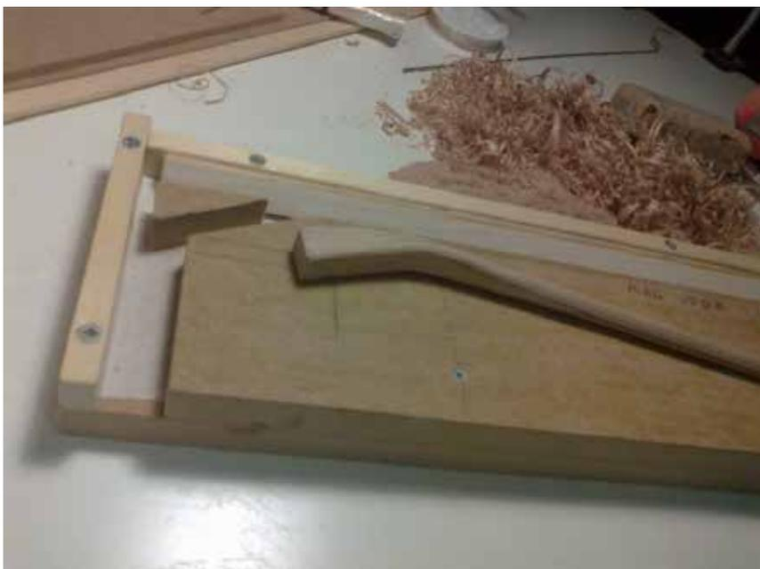
For the frog I have made an oblong hole in the bow, by moving a cutter with a mechanical stage over the fixed bow.
