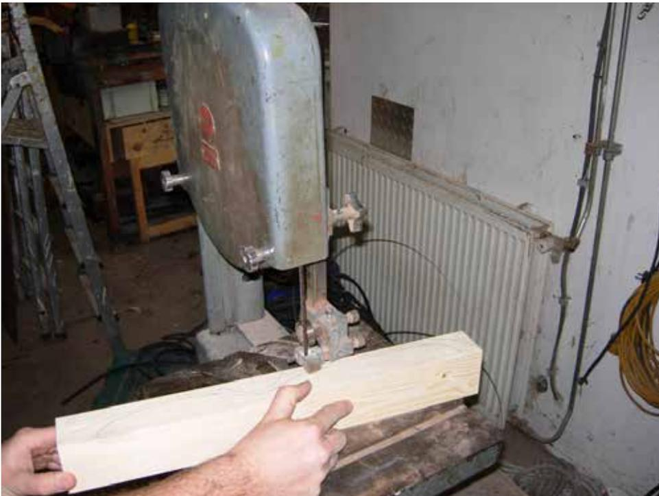
To solve this some curves were cut out from two sides. It proved difficult to match cuts made from two sides. Then there is a lot of finishing with chisels, files and sandpaper needed to get everything in order.
