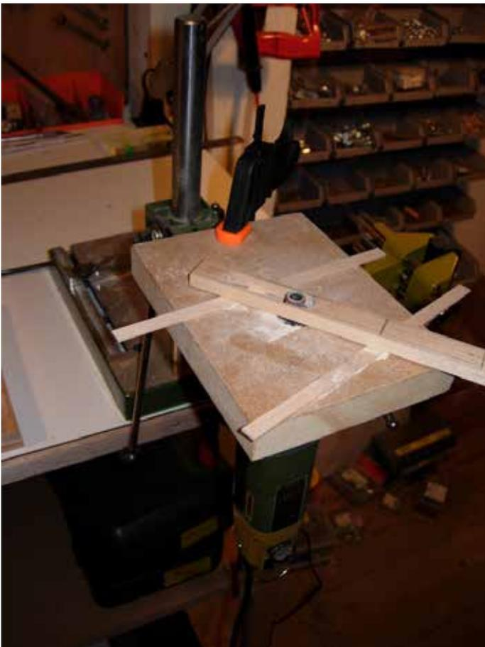
With this tool, I could also cutter the outside of the keys in the desired form.
