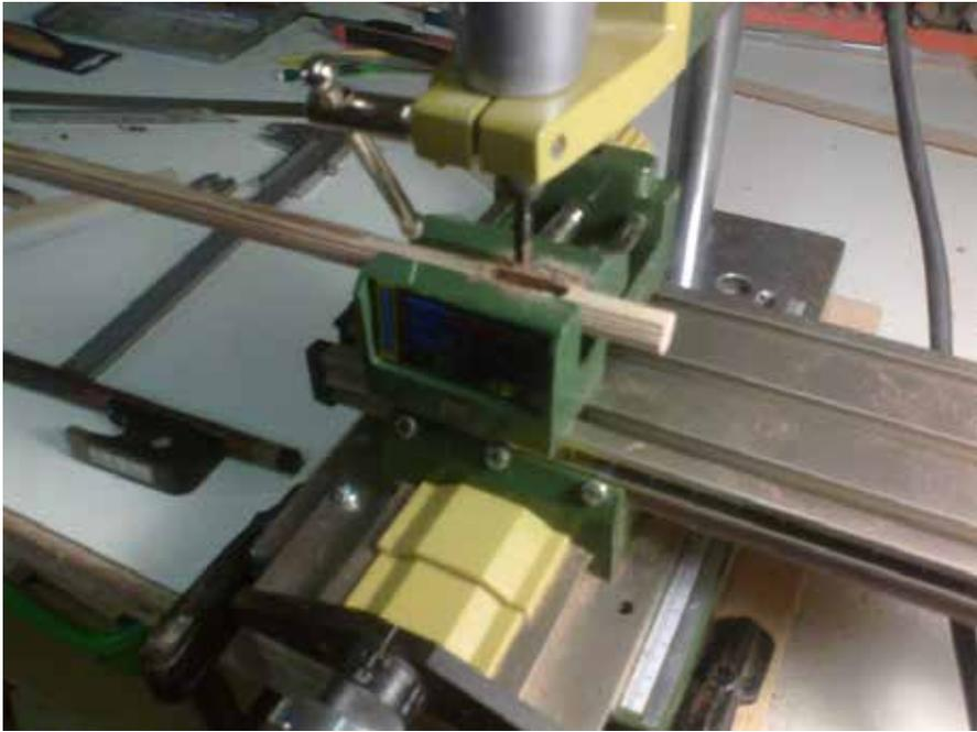
At the tip of the bow, I have glued an ebony block with square hole in it. This hole is for fastening the bow hair. The next picture shows how I have drilled a square hole by drilling away the edges of the hole and by filing.
