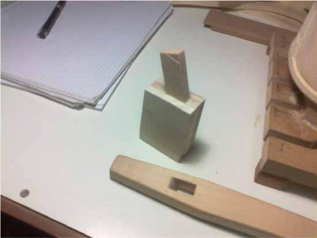
The holes for the sympathetic strings should run through the middle of the front of the tailpiece to the bottom of the cut that is made for the ends of the strings - a slight angle so. I have solved this by tilting and clamping the tailpiece to the workbench and drilling vertically.
