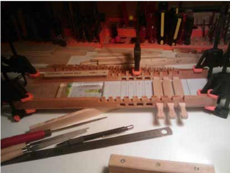
I glued thin leather on the MDF piece under the lower the key guides. The key guides were clamped to the MDF piece. That made little adjustments possible.
