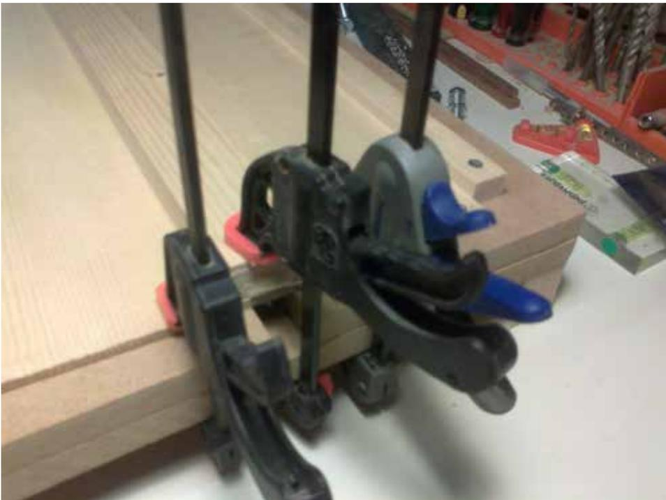
With the template I could exercise horizontal and vertical pressure. I attached adhesive tape to the edges of the top plate to protect the wood against glue. The mould had a notch below the bond line which gave room for the expansion of the glue.
