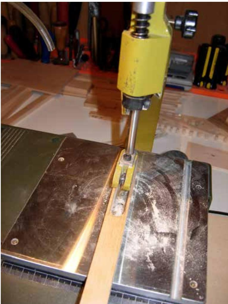
I thought it would be better to cutter the keys. To do that and I have turned a micro drill into a router table below. That was pretty simple: 1) by turning the micro drill holder upside down and 2) by fitting a custom-made small plateau which the cutter sticking up.
