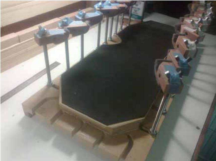
The harpa body can be placed in it and the top plate can be glued and clamped with 25 clamps. Before applying glue I attached adhesive tape on places where glue might damage the wood.
