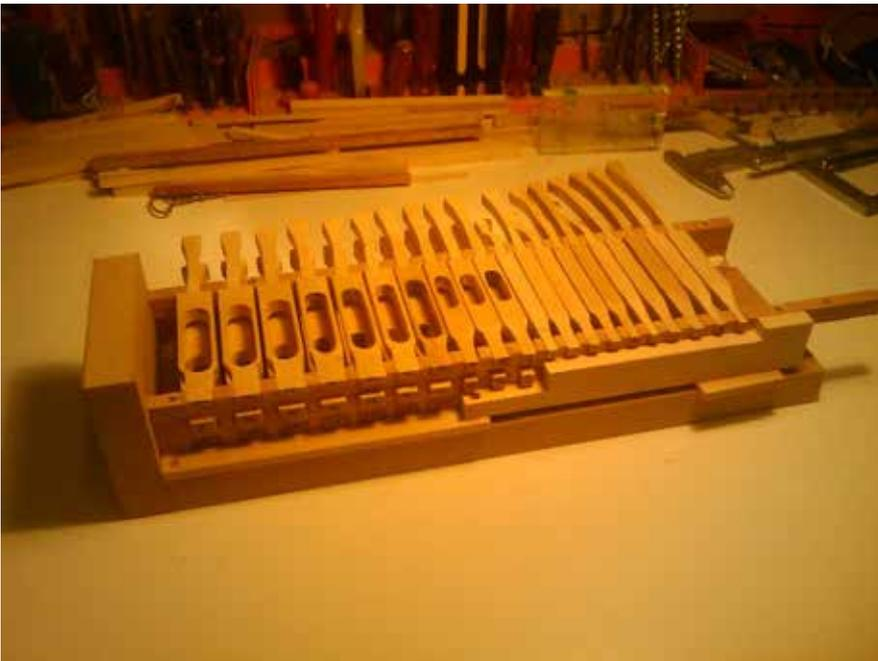
The vertical block at the left side of the key box is a temporary replacement for the nut over which the strings will run. It is an easy tool to place on the keys exact marks for placement of the tangent (holes). The holes in the keys at each layer have a different diameter. I drilled them with a drill press.
