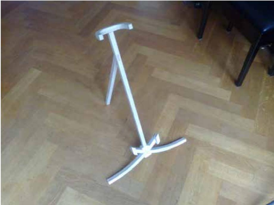
The picture above shows what I've made. The standard consists of five parts which click together without screws: two round legs that click together, a vertical support for the harpa that clicks around the legs, a back support which is attached to the vertical support with a wedge, and a safety bracket which is clicked on the vertical support. All parts coming into contact with the harpa have been covered with felt (not in this photo) to prevent damage to the harpa.
