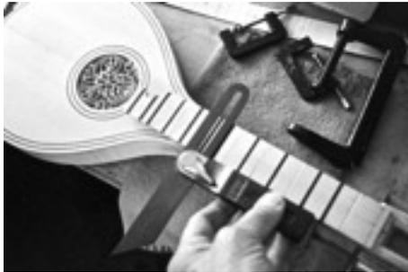
The slots for the frets are recut. It will be necessary to have a saw which is the correct size for the frets. Instructions on saw-sharpening easily found online will include adjusting the width of the cut. Now is an opportunity to check and if necessary, adjust the accuracy of the previous marking and cutting.
