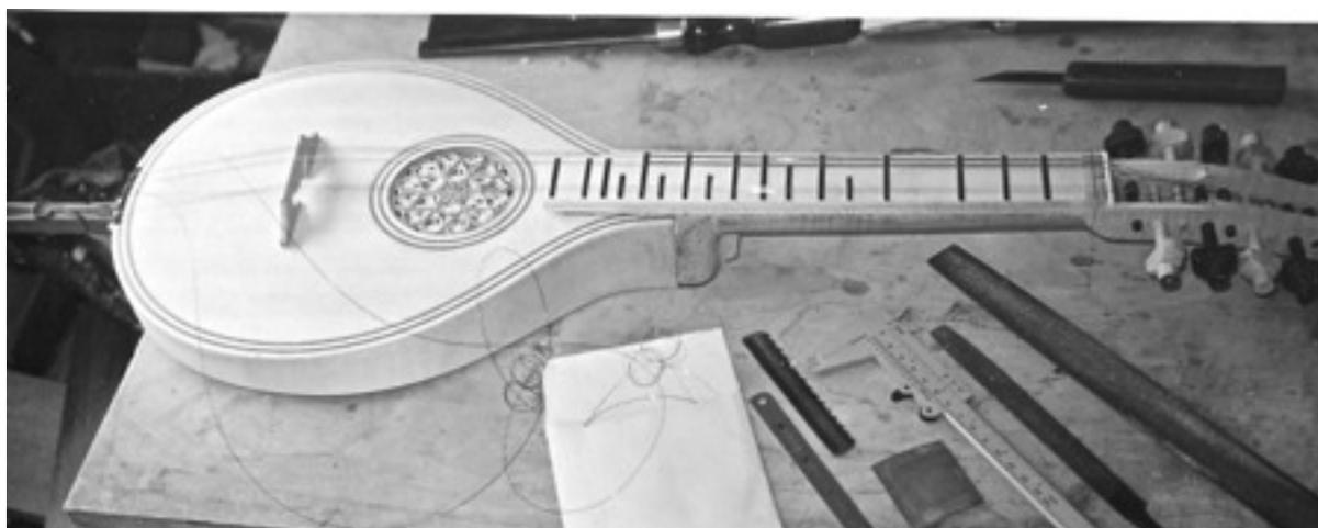
When fitting strings, especially as here where previously used strings are being reused, an ordinary wooden clothes peg truncated to a square end makes a useful third hand. Also in the photo are scraps of hacksaw blade reshaped to make scrapers for the slope up to the frets. The 'o' fret wire is at its theoretical 'nut' position.
