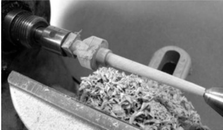
The rough-turned pegs can be taken towards completion. The photograph shows my method of ensuring that they can be replaced exactly in the lathe. They are being held by pressure and for longer or narrower pegs it would be better to use a three-jaw chuck in the headstock.
