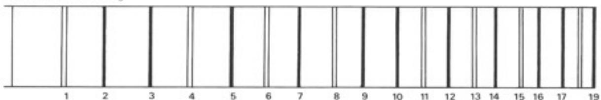
The slots for the wedges could be cut with a modified saw to give a constant depth. I make them freehand, aided by a small mirror behind the fingerboard as in the photograph. The side of the slot which will be occupied by the fret itself is cut at an angle, the other side at right-angles to the surface. Partial frets can be started with a saw, and finished with a knife.
