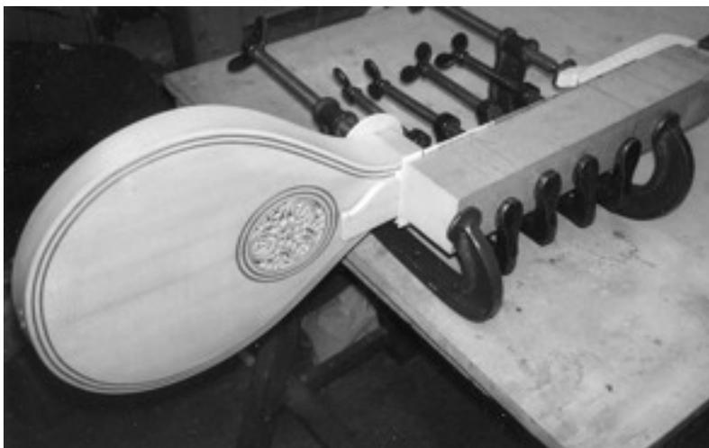
Playing the cittern will be helped by a low action and this can be aided by hollowing the surface of the fingerboard, technically to a very shallow parabola - in practice simply by scraping to a slight but even curve, about 0.5 mm deep on a 43/45 mm string length. This can be judged by a light behind a straightedge.
