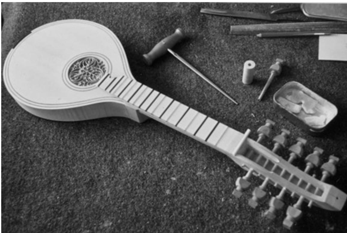
I don't finish the knobs of the pegs, nor fully fit them, until after varnishing in case they need to be returned to the lathe, or there are varnish splashes in the peg-holes which need to be reamed away. Talcum powder (not chalk, which is abrasive) and dry
