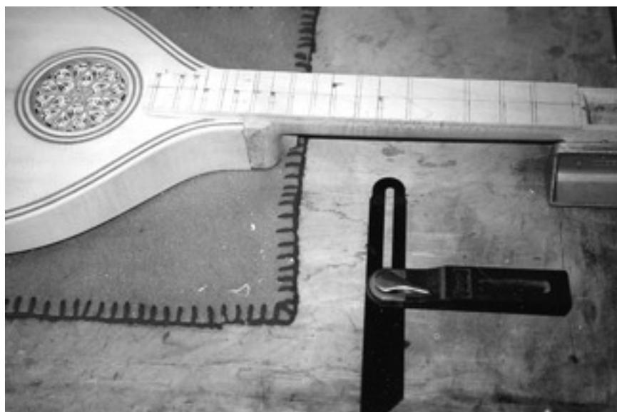
The fret positions are now marked along the centreline. I have various lengths of formica marked for different string-lengths and degrees of mean-tone. Marking the frets themselves at right-angles to the centreline will either require an adjustable square, or that the fingerboard has not
