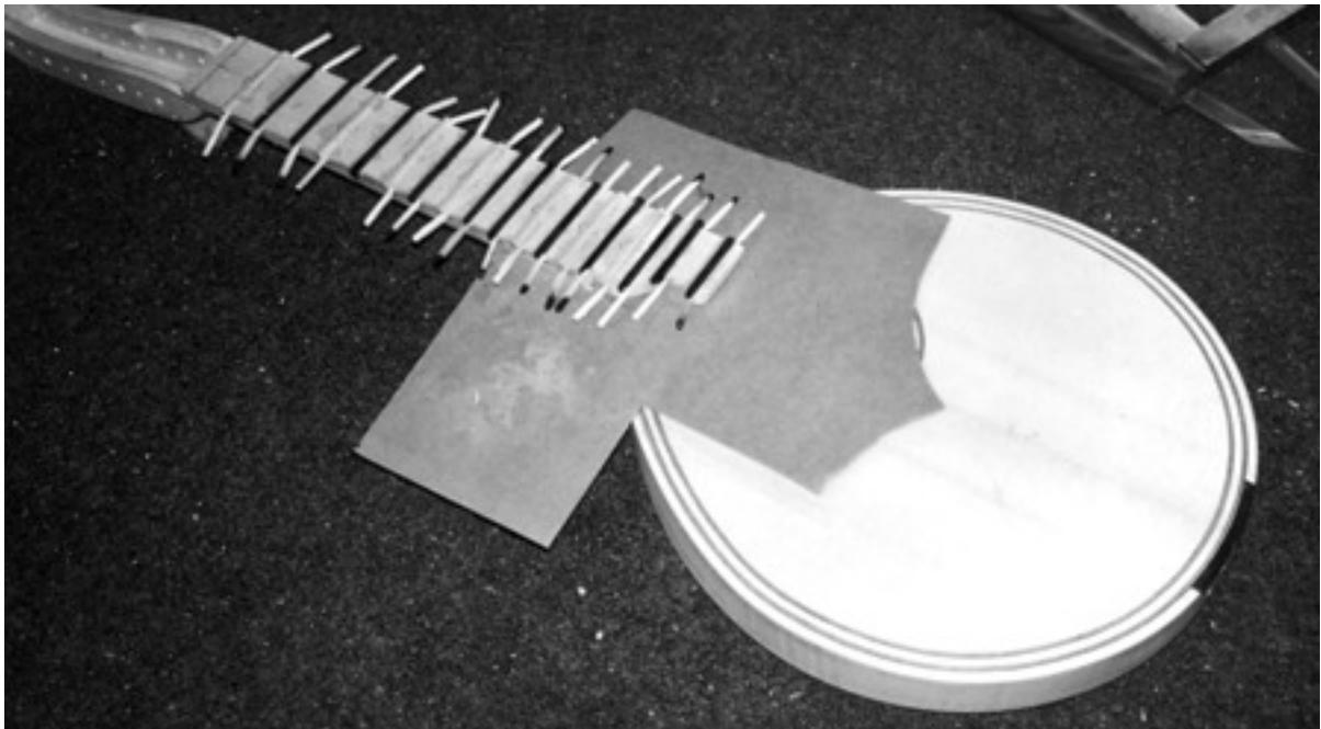
of what they were originally called. Their end-view of a half-dovetail (a full dovetail on one Italian instrument) is wedge-like, but experimental actual 'wedging' caused the fingerboard and neck to bend backwards... Occasional wedge shapes on original instruments are probably due to repair. It would be possible to retain a parallel appearance and form a wedge by tapering the depth. This has perhaps been done on
