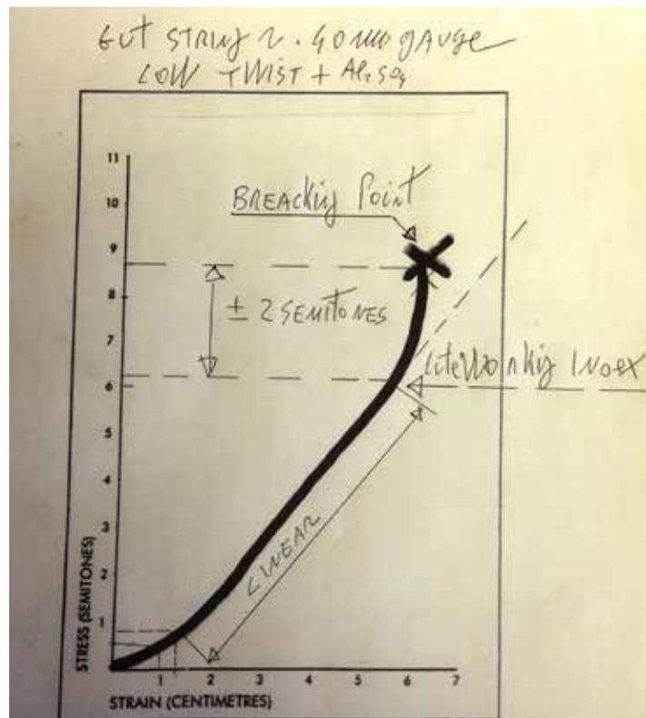
The string therefore maintains its linear stretching behaviour until about 2-3 semitones from the breaking point; beyond this value, it enters the critical phase. This is different from the typical behaviour of metals and nylon/nylgut/fluorocarbon strings. From this point gut almost completely loses its ability to stretch itself reaching rapidly its breaking point.
