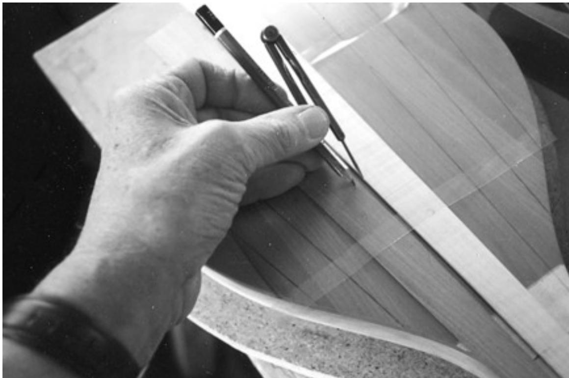
substitute. A bendable straight-edge - a metal rule or strip of formica - will be necessary. How accurate the joint will be can be judged by holding the strakes up to a strip-light or a window. The thickness of the back means that ornamental lines, if
