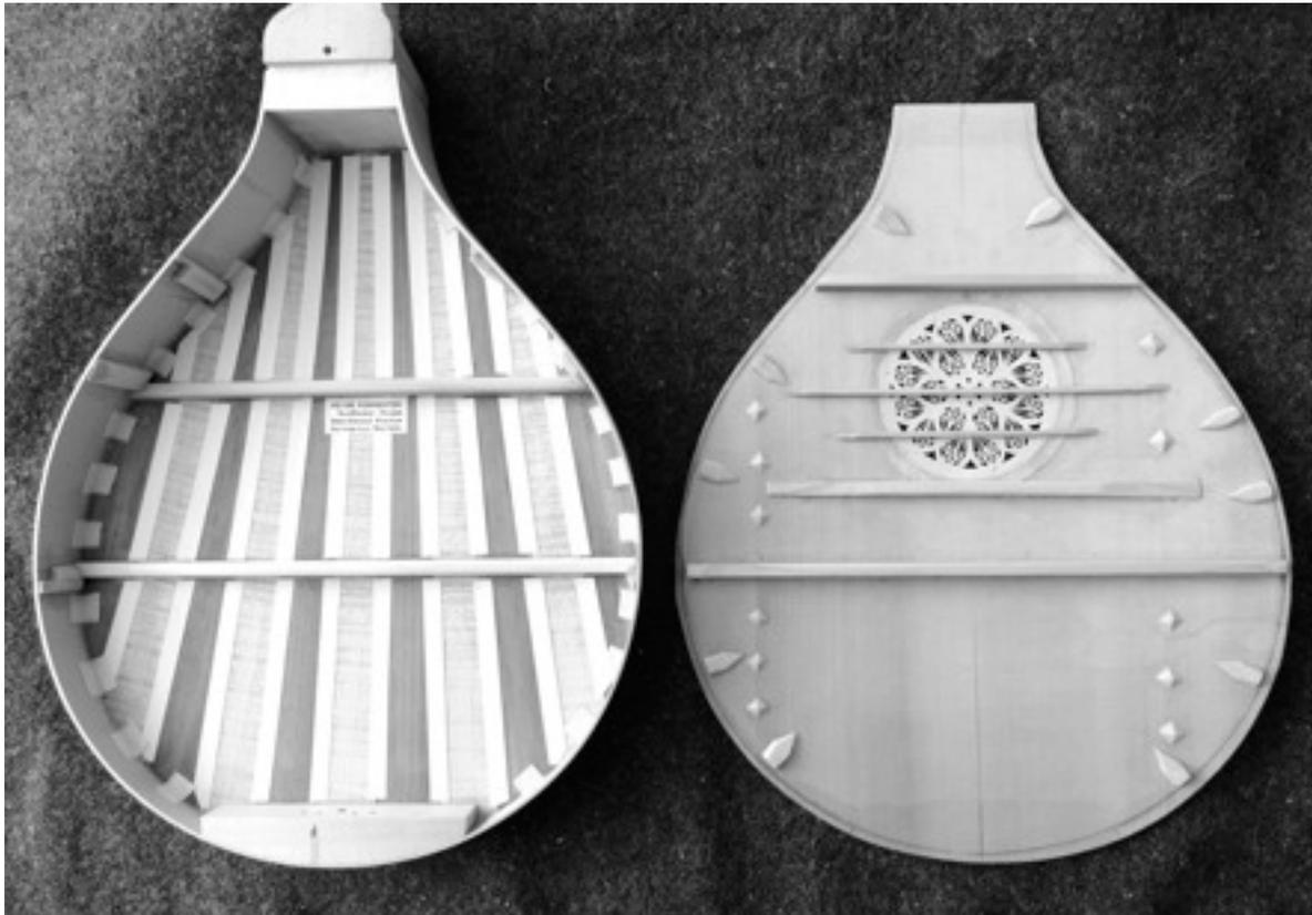
The two back bars are at the widest part of the body and below the centre of the rose. The main belly bar is above the back bar and is prevented from collapsing by small reinforcing supports which connect these bars. Further reinforcements are associated with the other back bar and with the belly bar above the rose. Their purpose is to strengthen the flattish areas of the sides against the downward pressure of the
