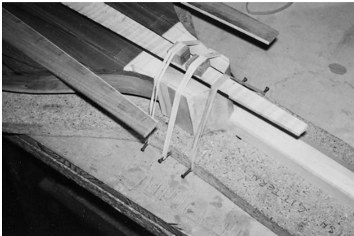
used, need to be cut from sheet veneer and glued to each strake before the latter are glued to the neck-block. After checking that these lines have not altered the fit between strakes, the central strake is glued to the block. The photo above shows a simple clamping method which is quicker and easier than G-cramps. If there is more
