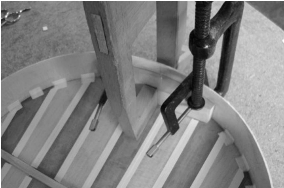
small chamfer on the edge of the block. Be sure that the block is sufficiently deep on its inside surface. Gluing and cramping up should be straightforward. Cramp to the side first, then to the back.
