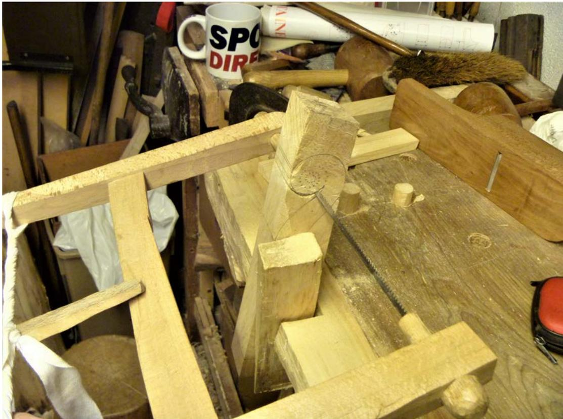
Fig. 6. The vice notch in action. A violin scroll being sawn. (Apologies for the historically inappropriate tea mug in the background.)
