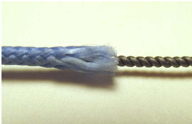
Exposed Two Strand Twisted Core
