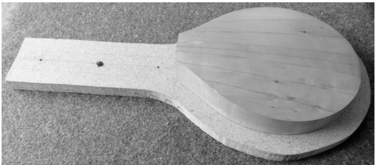
The mould can be solid or made in layers. Both work, but it is convenient to be able to use small cramps or clothes-pegs to hold the back staves in place while the glue sets. The curves and flats across the back are made much like a lute back. Their slighter curvature is a little more difficult to make accurately.
