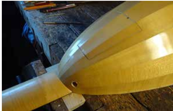
The soundboard has been replaced and the mic located inside the lute.
