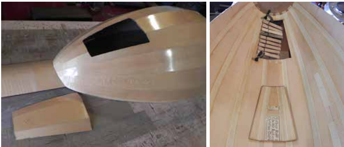
The hatch cut out of the body—the removed wood becomes 'The Hatch Cover'
