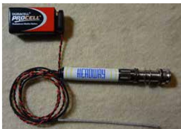
Headway's miniature pre-amp, jack socket, Snake and battery.
