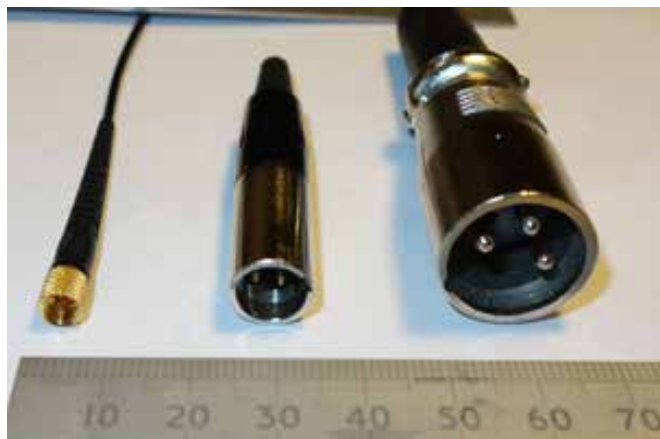
Three types of connector: on the left, the new Microdot, in the centre, a mini-XLR, on the right, a standard XLR. These are all jacks and they plug into comparable sockets.
