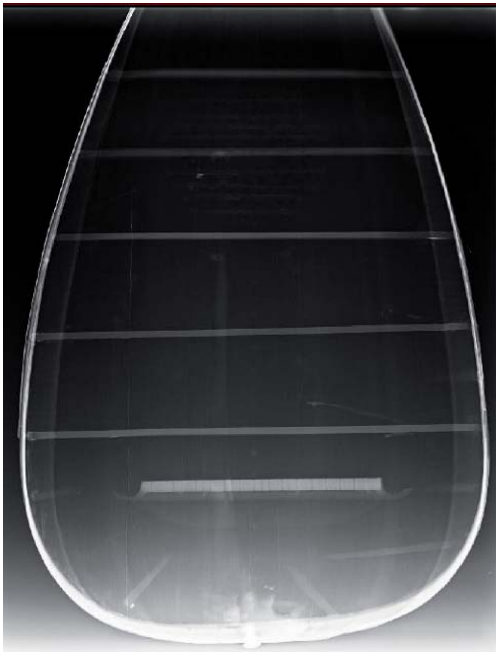
FIGURE 7: X-ray image of the Tielke 1698 angélique, body with bridge and lower bars.
