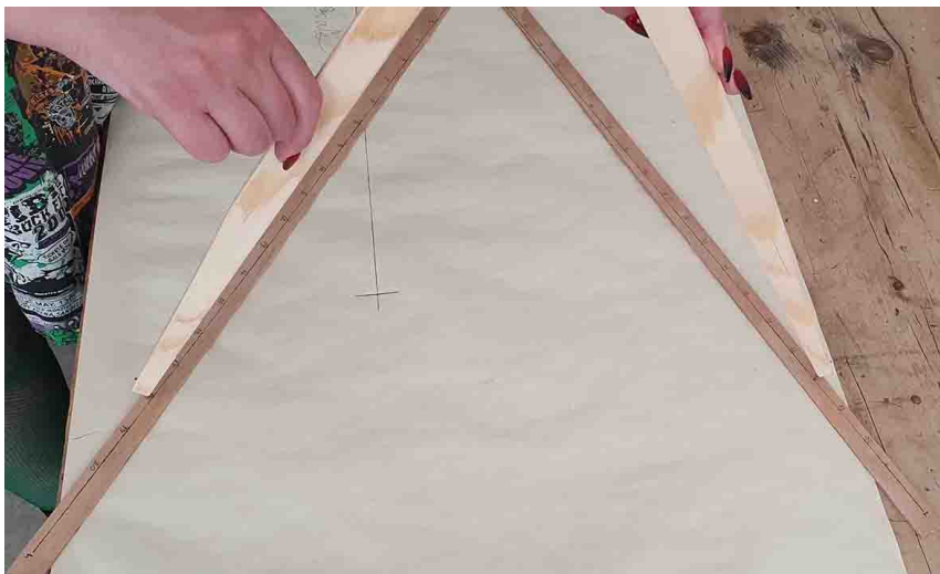
Plate 3: Transferring a reading to Sector marks at '18'. The Sector should be on a flat surface to allow adjustment and accuracy.
