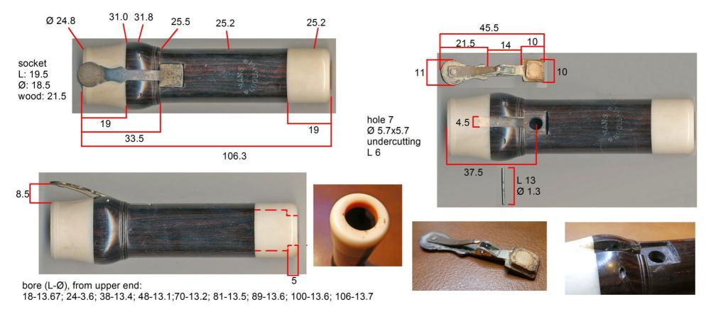
pitch: about a1=415 Hz (according to Hans Coolsma: 415 to 419 Hz)
