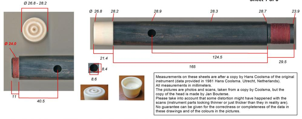
Bore of the head of the copy: Ø 19.3 from cork end to L 130, and Ø 19.2 from L 130 to lower end; cork at about 18 mm from mouth hole centre. Original bore c. 19.5, cylindrical.
