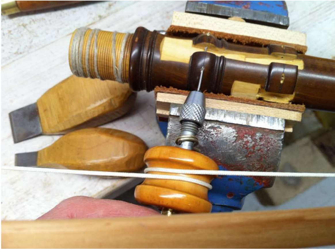
The key pin hole drilling process, using a bow drill.
