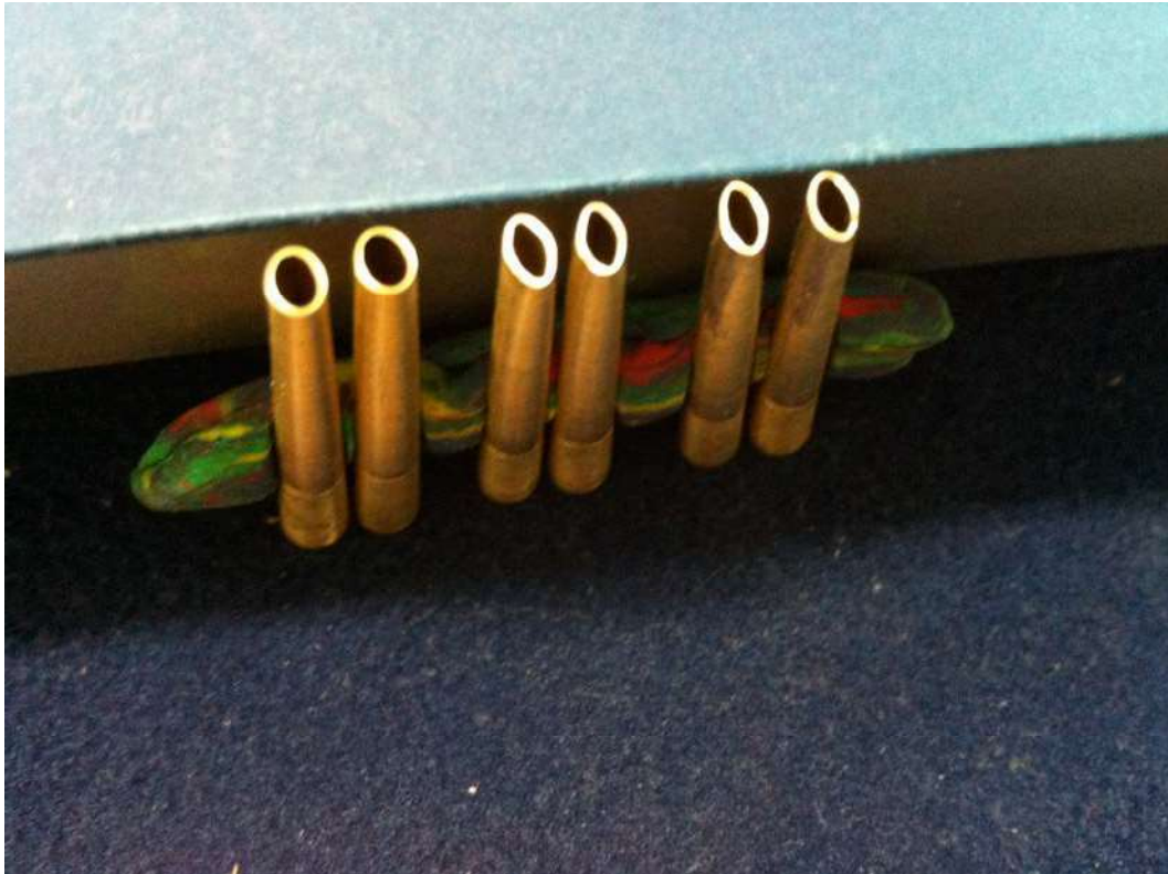
The angle visible from the side view, and the resulting ovality from the top view.
