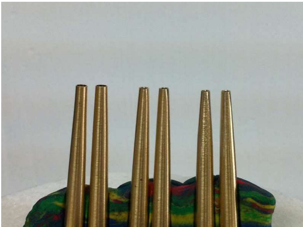
Three pairs Chiarugi staples: unaltered; hammered (to increase the ovality); filed as well to thin the sides near the tip and to increase the angle.
