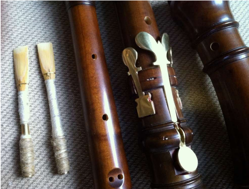
The holes have not been darkened yet and still need some finishing on the edges; 2 reeds with 50mm and 58mm long staples.
