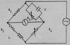
For balance  $R_1.R_4 = R_2.R_3 = L/C$
